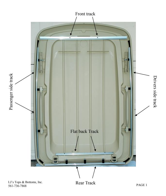
Sides & Rear tracks— Install clip nuts over pre-drilled holes in tracks so that the nut part of clip is on the same side as the opening in tube.
