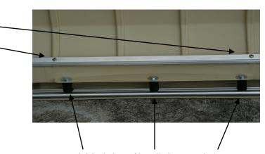
Finished view of installed rear track. See picture below for drilling instructions. After holes are drilled slide fender washer onto 2 1/4" bolt insert through hole from inside of top, then add a 1/2" and 1" spacer to bolt. Secure to track.
