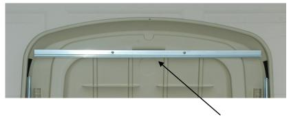
Front Valance Track—Slide front valance onto track so that good side of valance and flat side of track face forward. Secure track by using the 2 existing holes in top with sheet metal screws included in the kit.
