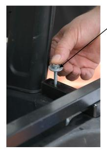
Place the Bag Par-Tector cross member on top of the bag rack aligning the holes up with the newly installed metal inserts. Then secure the Bag Par-Tector cross member with the supplied 1/4" bolts and washers.
